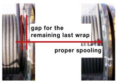
Fig. 41: proper spooling of first layer in order to avoid gaps to shim-plates that can cause rope crushing
