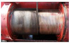
Fig. 29: drum ground should be visible for proper measurement
