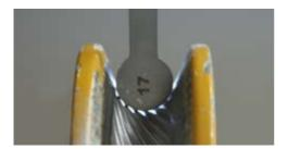
Fig. 21: negative impression of a used sheave
