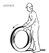
Fig. 2: proper unwinding off a coil
