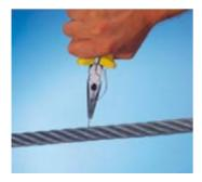
Fig. 36: How to remove an distant wire
