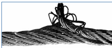
Protrusion of the steel core, generally linked to basket deformation. This rope must be replaced immediately.
