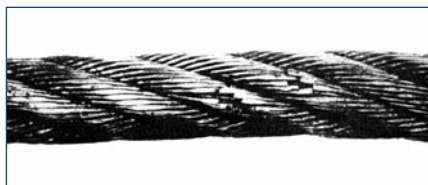
Broken wires in two strands due to bending fatigue, linked to major localised wear. This rope must be replaced.
