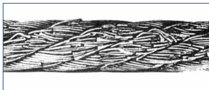
Major wear and high number of broken wires in a regular lay rope. This rope must be replaced immediately.
