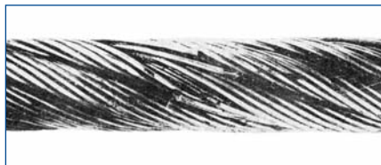
Broken wires in a single strand and slight wear in a lang lay rope. In this case the broken wires must be removed to make the rope smooth.
