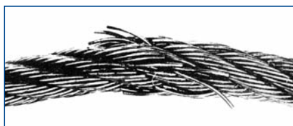
Broken wires in several strands, close to a return sheave (sometimes hidden by the sheave). This rope must be replaced.
