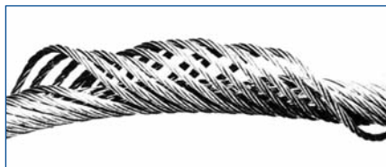
Birdcage in a multilayer (non rotating) type rope caused by forced rotation around small grooves or excessive fleet angle. This rope must be replaced immediately.
