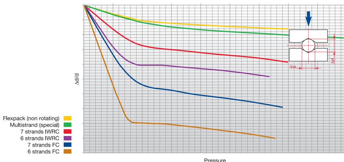
For each curve, two main areas can be identified: the main ratio of the diameter variation is obtained during the first stage of compression, while after having reached a certain deformation value, the diameter variation slows down and the curves show similar slopes.
