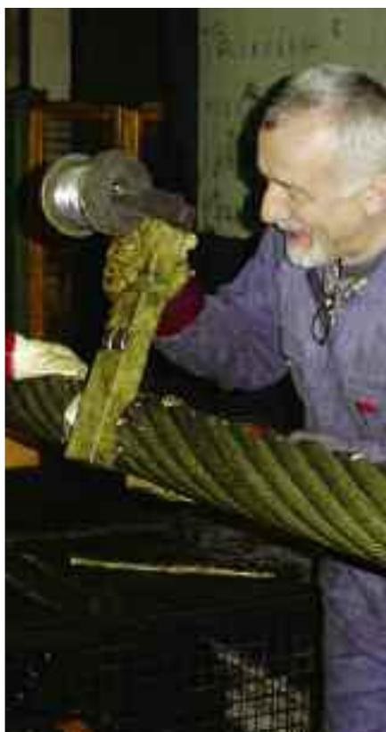
**For the cut end of six strands ropes, two servings each of a length at least six times the rope diameter should be used.
