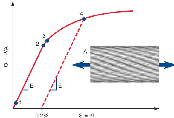
Each wire rope is designed to operate in a certain range of the linear portion depending on the required safety factor. High safety factor means that the rope will work in the lower range of the linear area, while low safety factor means that it will work closer to the yield limit.
